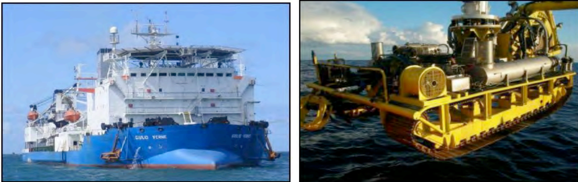
Figure 2-5 Examples of Vessels Required for Offshore Cable Laying
