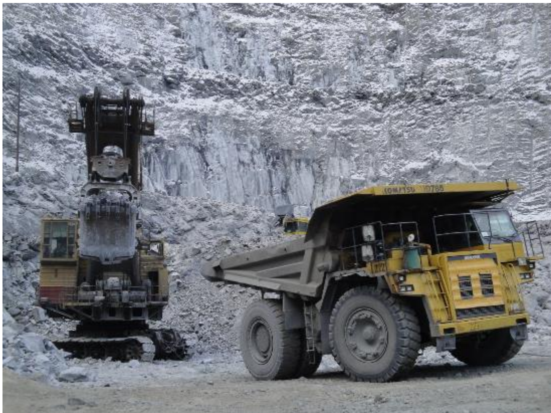
Figure 7: Example of excavator loading a haul truck in an open pit
