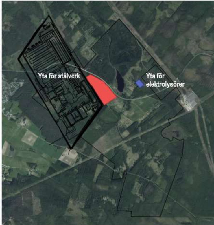
Figure 8-7 Estimated surface area for surface water management. The surface water management from the steel works surface is marked with red and the surface water management with electrolyzers is marked with blue.
